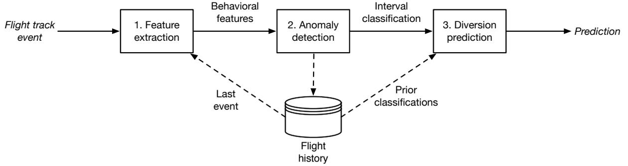
Figure 1: Overview of the prediction model for diversion detection
