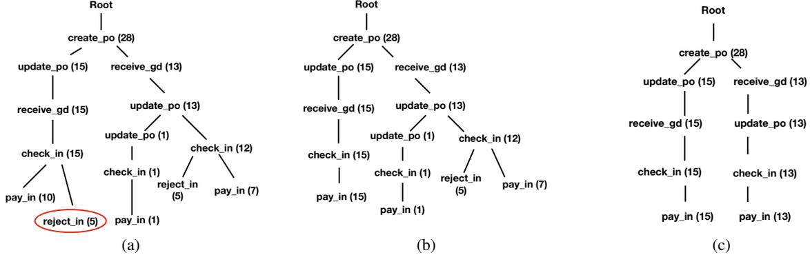
Figure 1: (a) Prefix tree of the example; (b) tree obtained after pruning the highlighted node and reconstructing the tree; (c) final tree returned by PRETSA for the example, setting  $k = 8$  and  $t = 1.0$ .
