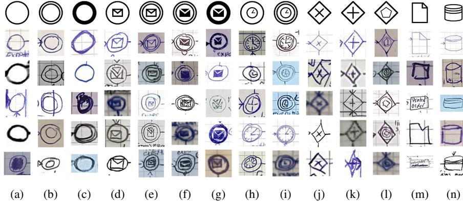
Fig. 8: Examples of hand-drawn *events* (start 8a, intermediate 8b, end 8c, message start 8d, message intermediate catch 8e, message intermediate throw 8f, message end 8g, timer start 8h, timer intermediate 8i), *gateways* (exclusive 8j, parallel 8k, event-based 8l) and *data elements* (data object 8m, data store 8n).
