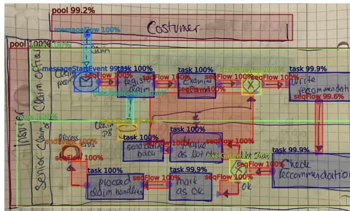
Fig. 3: *Step 1*: Candidate shapes and edges have been classified and localized through bounding boxes, in addition edges have predicted arrow head (▷) and tail (◁) keypoints.
